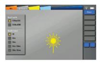
Invisible light source (1310/1550nm) can provide the following sources of light: CW, 1kHz, 2kHz modulated and 1kHz & 2kHz blink.
